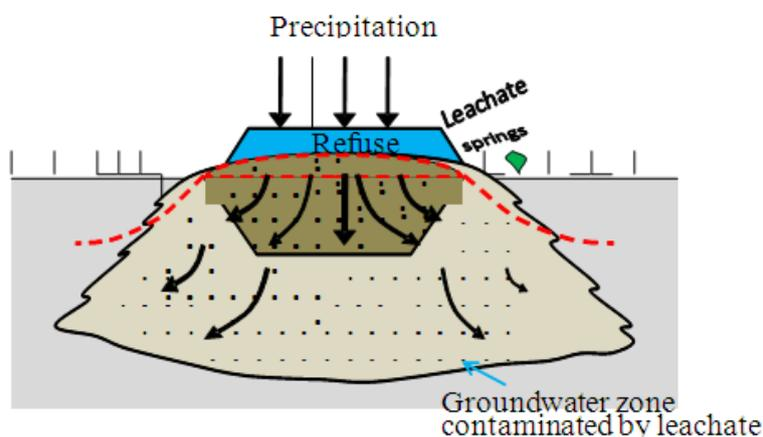
*Figure 1: Conceptual diagram of leachate migration from a landfill*
