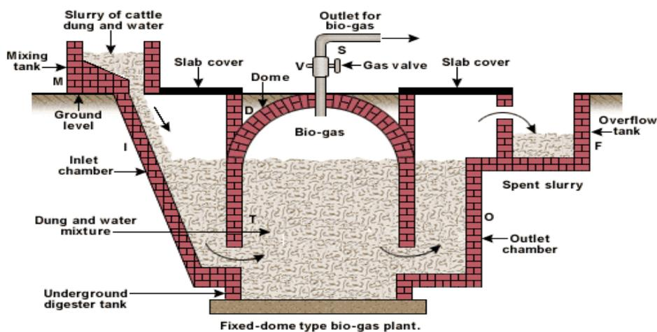
Fig1: Fixed Dome Biogas Type
