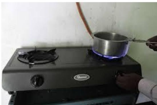
**Fig 3: Biogas used as Gas Cooker**
