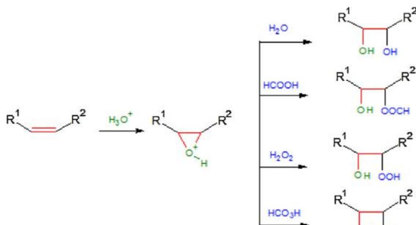
Figure2: Cycle opening reactions
