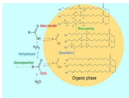
Figure3: Simplified mechanism for fatty acid epoxidation.
