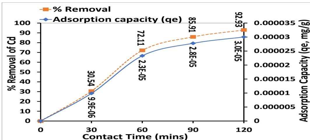
Figure 13: Effect of contact time removal of Cd in mine water
