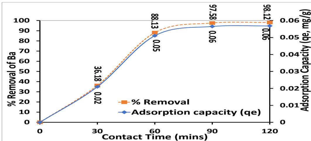
Figure 12: Effect of contact time removal of Ba in mine water
