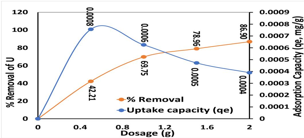
Figure 1: Wood ash Adsorption Dosage Treatment of Uin Gold Mine Water
