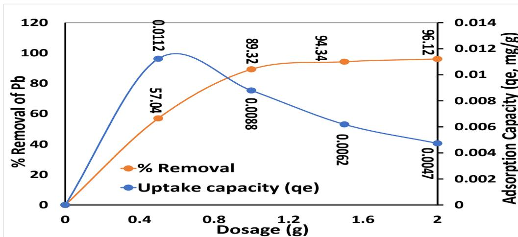
Figure 5: Wood ash Adsorption Dosage Treatment of Pbin Gold Mine Water
