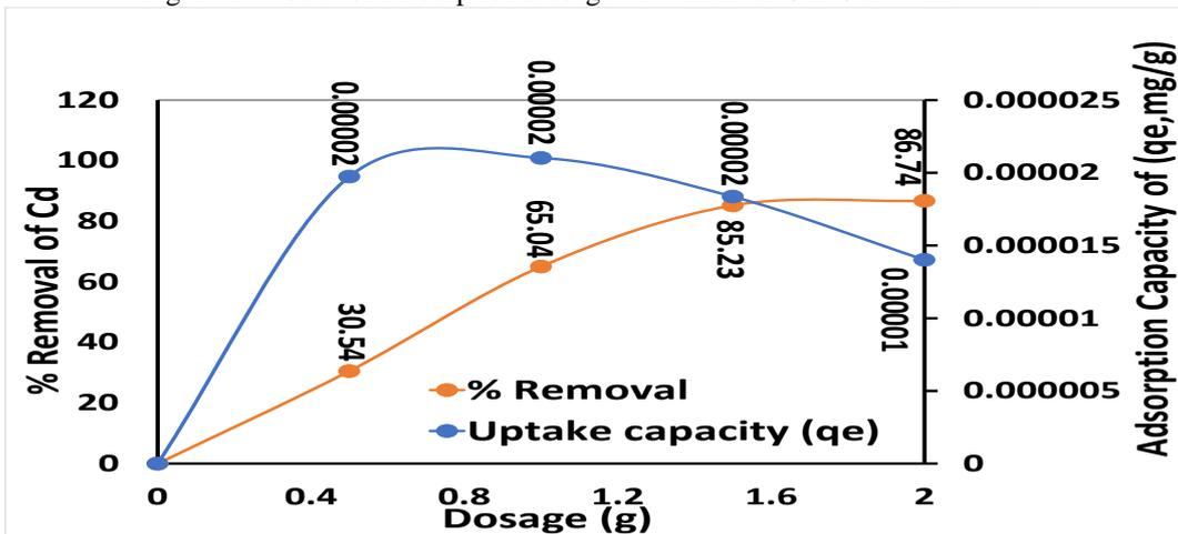
Figure 2: Wood ash Adsorption Dosage Treatment of Cd Gold Mine Water
