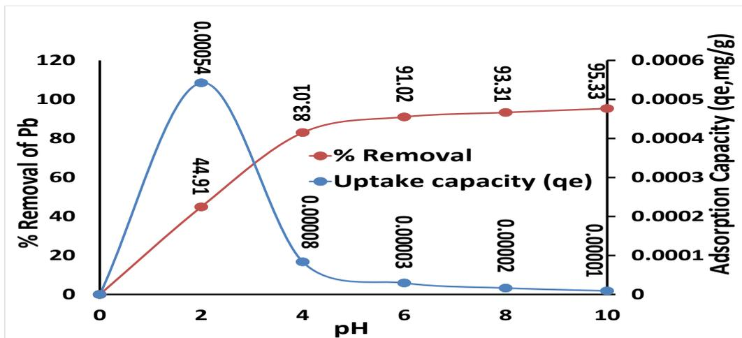
Figure 10: Effect of pH on Wood ash Adsorption in Gold Mine Water
