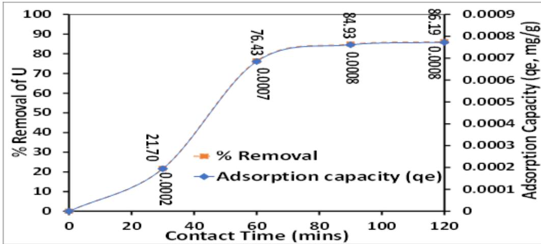
Figure 11: Effect of contact time removal of U in mine water
