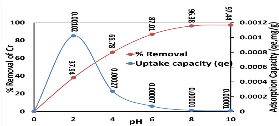
Figure 9: Effect of pH on Wood ash Adsorption of Cr in Gold Mine Water
