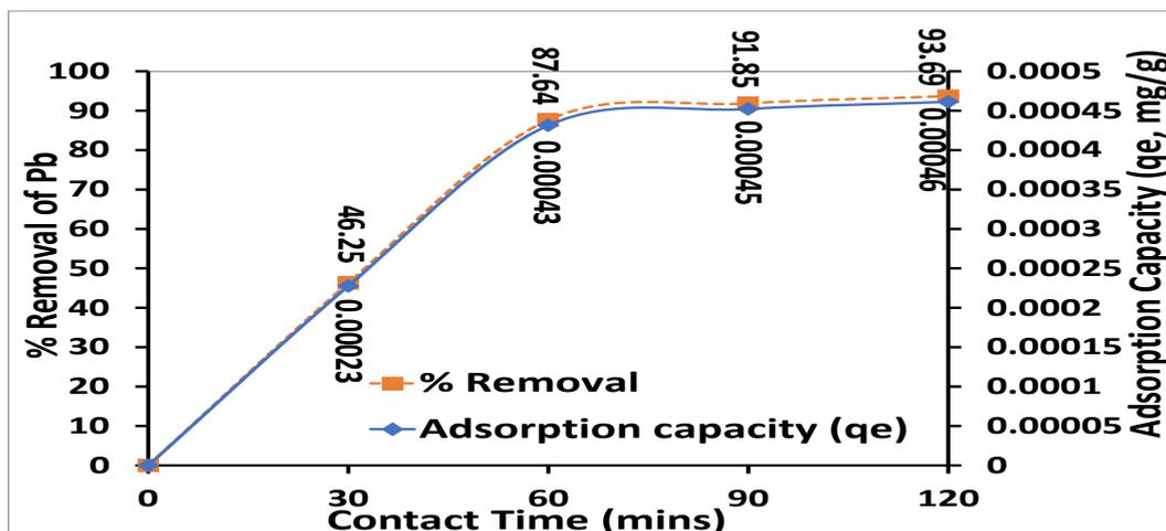
Figure 14: Effect of contact time removal of Pb in mine water
