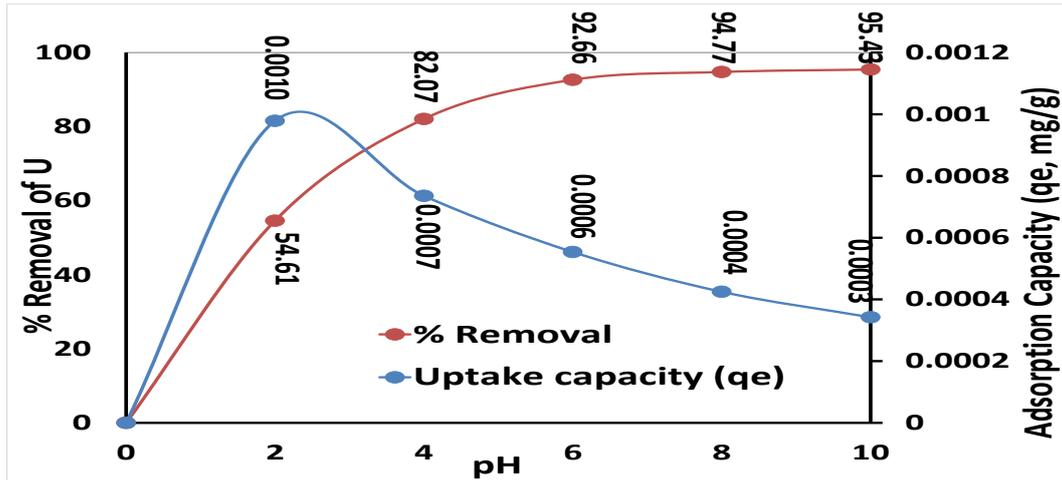
Figure 6: Effect of pH on Wood ash Adsorption of U in Gold Mine Water
