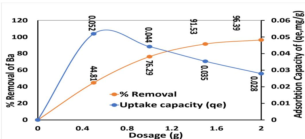
Figure 3: Wood ash Adsorption Dosage Treatment of Barium In Gold Mine Water
