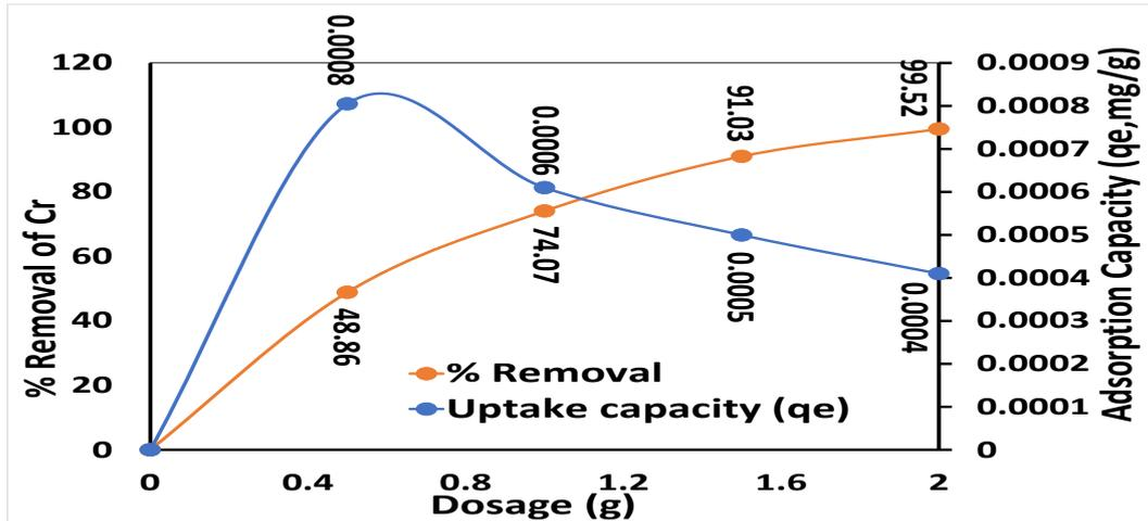
Figure 4: Wood ash Adsorption Dosage Treatment of Crin Gold Mine Water
