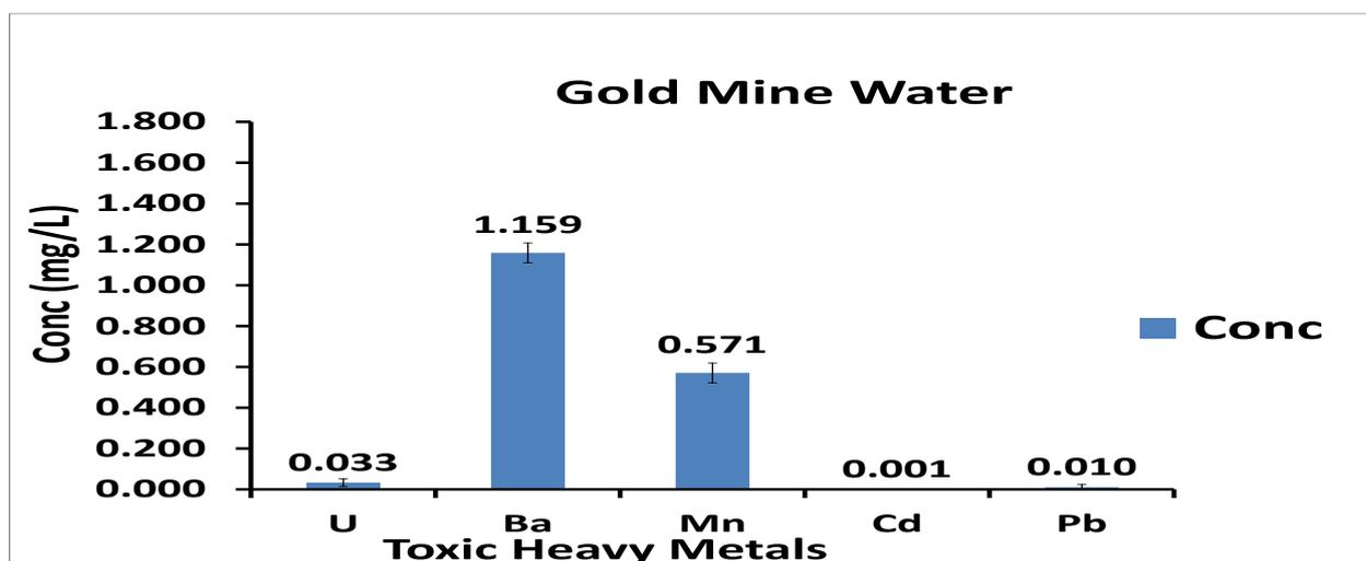
Fig 2: Toxic heavy metals present in Gold mine wastewater: (n = 3)
