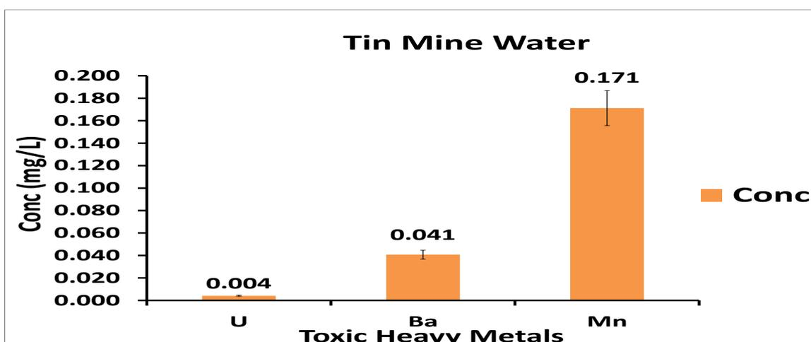
Fig 5: Toxic heavy metals present in Tin mine wastewater: (n = 3)
