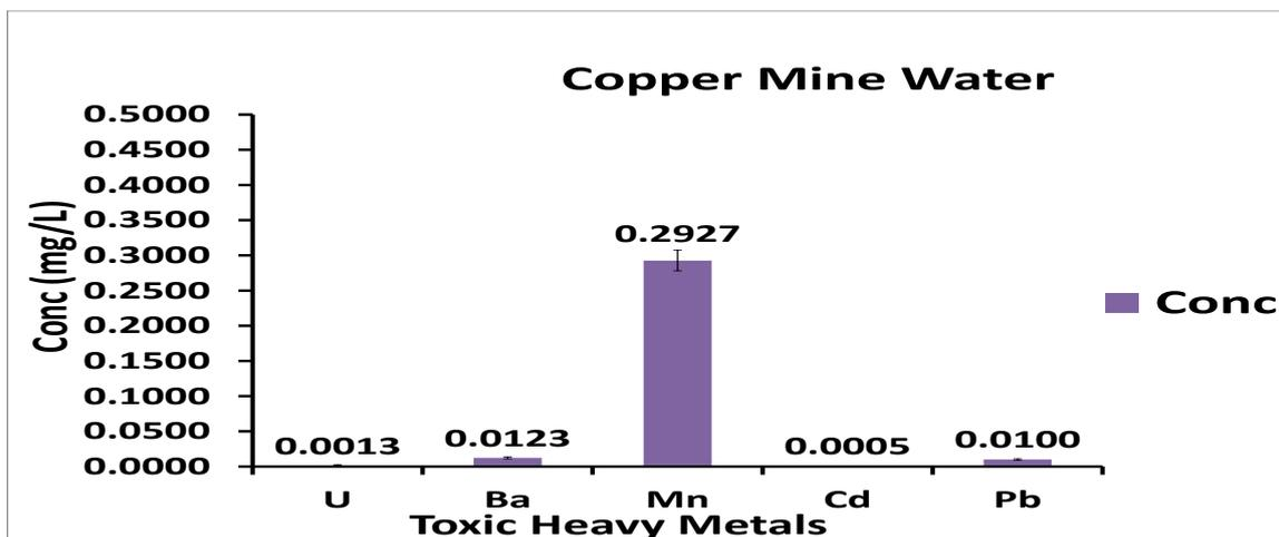
Fig 3: Toxic heavy metals present in Copper mine wastewater: (n = 3)
