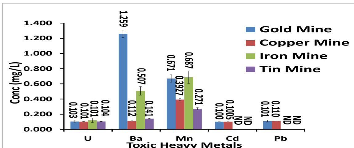
Fig 6: Toxic heavy metals present in four different mine wastewater: (n = 3)
