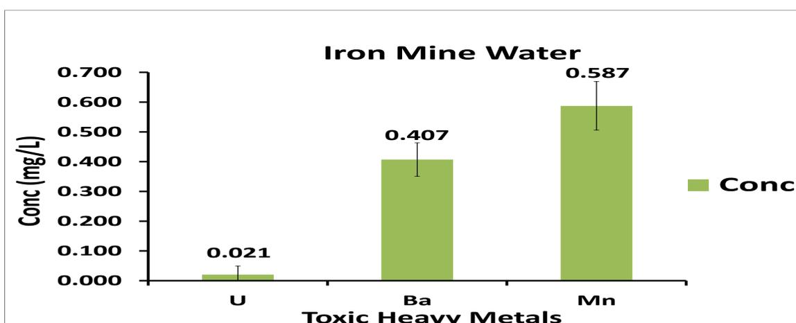
Fig 4: Toxic heavy metals present in Iron mine wastewater: (n = 3)
