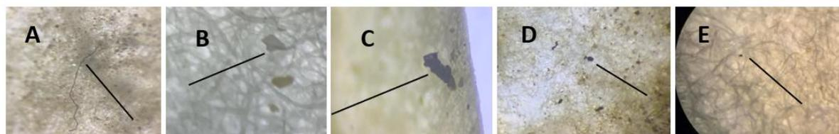
**Figure 2.** Types of microplastics observed in the sample: (A) Fiber, (B) Film, (C) Fragment, (D) Granule, (E) Pellet
