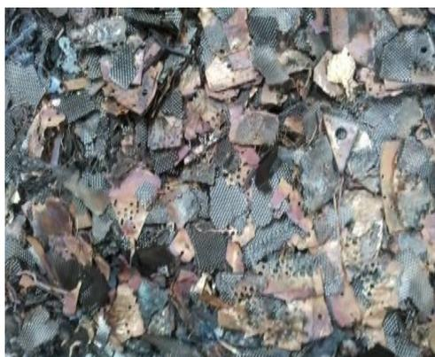
**Fig.3a.**PCB after incineration in muffle furnace
