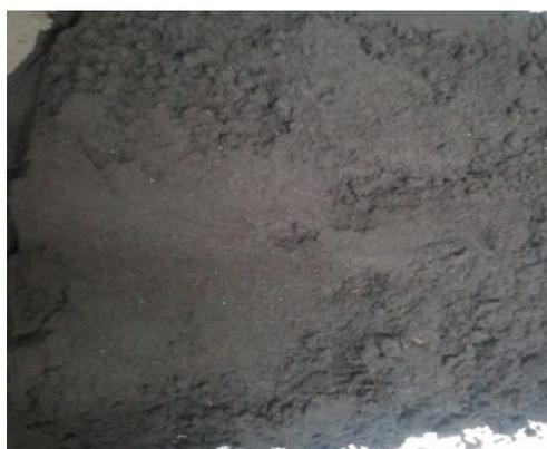
**Fig.3b** PCB powder of after incineration
