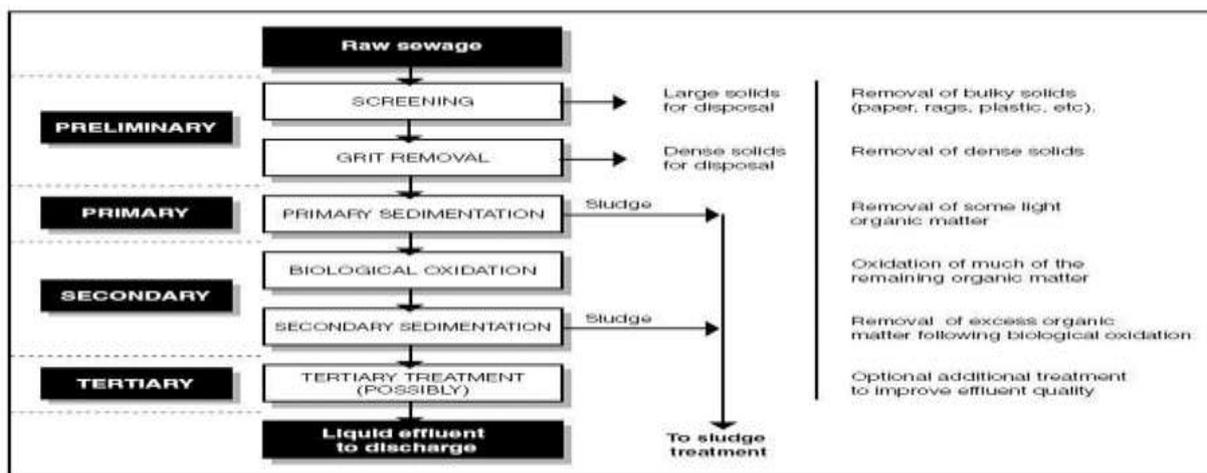
Figure 1. Typical stages in the conventional treatment of sewage
