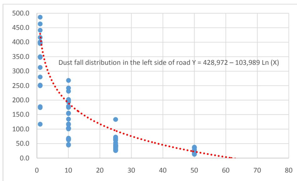
Fig. 6 Dust distribution in left sides of road
