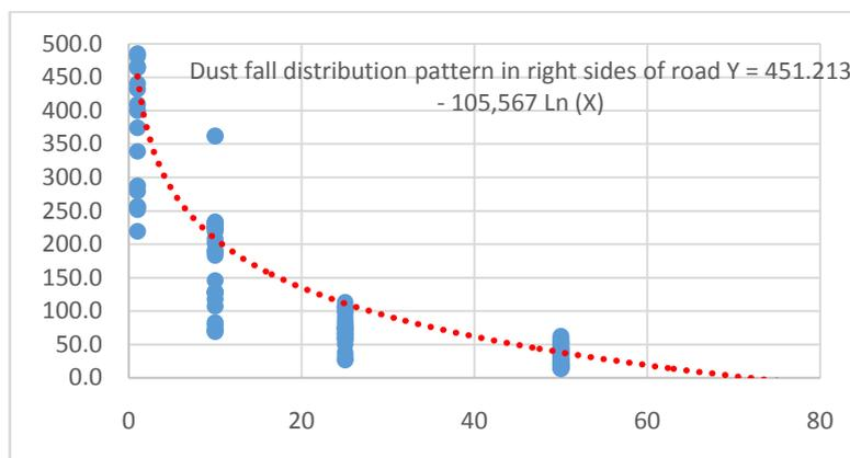
**Fig. 5** Dust distribution in right sides of road
