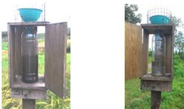
Fig. 2. Dust fall collector which was set up at point observation.
