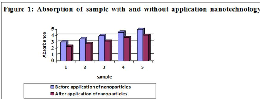
Figure 1 reveals that the absorbance of the samples has been noticeable reduction in fluoride. The study showed 24.50 % reduction in absorbance for sample having fluoride 3ppm fluoride content, 21.93% reduction for 3.5ppm, 13.64% reduction for 4ppm fluoride concentration, 11.07% reduction for 4ppm fluoride concentration and 7.62% reduction in absorbance for the sample containing 5ppm of fluoride.
