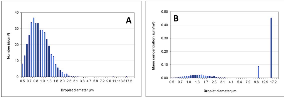
**Figure 2.** Droplet size distribution, (A) number and (B) mass concentration for the electrostatic spraying system during operation.
