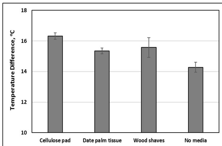
**Figure 5.** Temperature difference between inlet and outlet air for different porous wetting media
