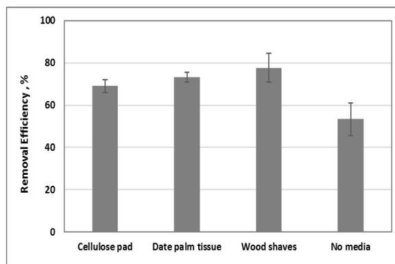
Figure 7. Dust removal efficiencies for different porous wetting materials while using a charged water spray.
