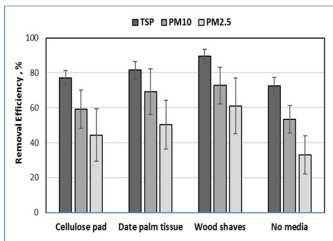
**Figure 8.** Particulate removal efficiency for the three particles sizes (TSP, PM<sub>10</sub>, and PM<sub>2.5</sub>) by the scrubber.
