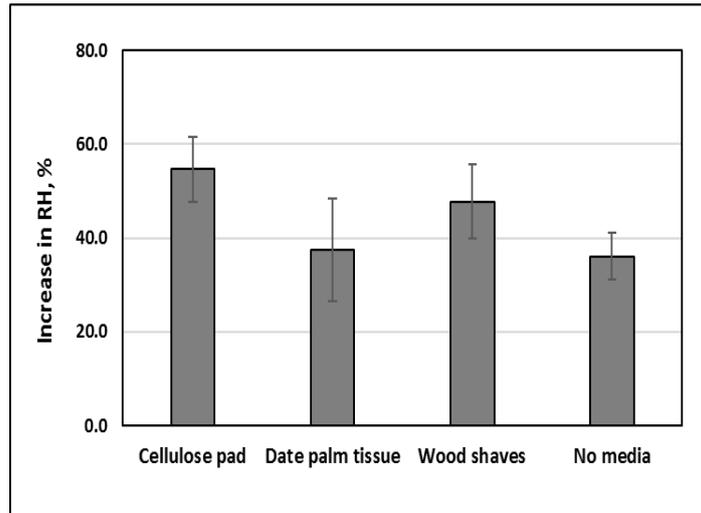
Figure 6. Relative humidity (%) difference between inlet and outlet air for different porous wetting media
