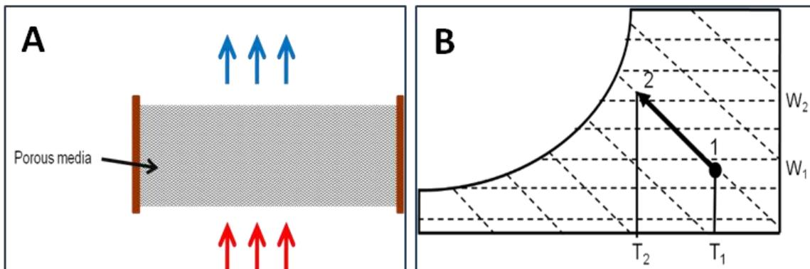
**Figure 4.** Schematic diagram of (A) air bath within porous wetting media, (B) evaporative cooling process.
