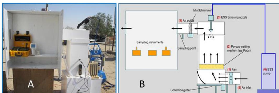
**Figure 1.** (A) Photograph of the test setup, (B) Schematic diagram showing the components of the air cleaning device (not drawn to scale).
