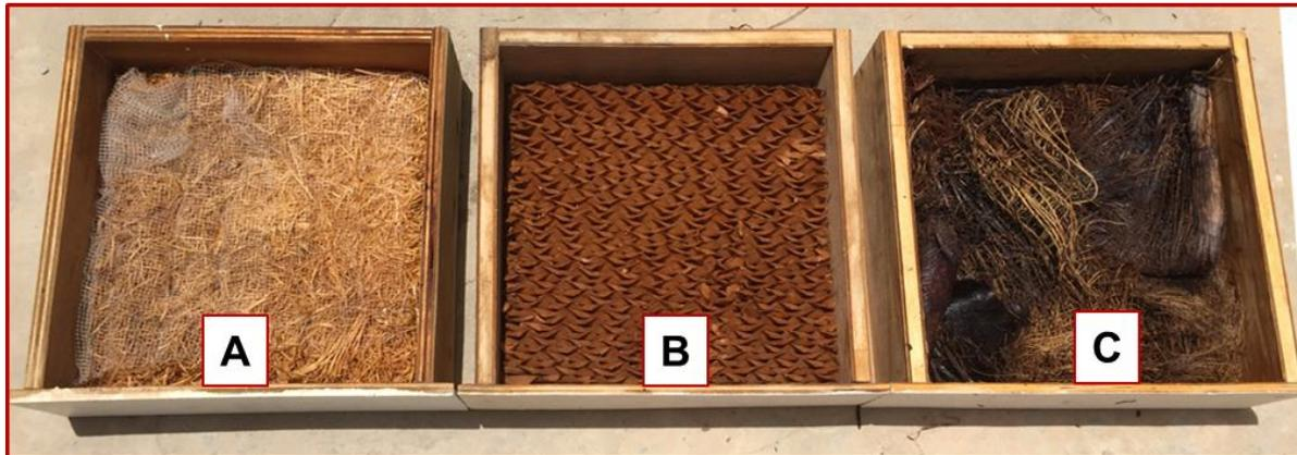
**Figure 3.** Porous wetting media used (A: wood shavings, B: cellulose cooling pads, C: date palm fibers).
