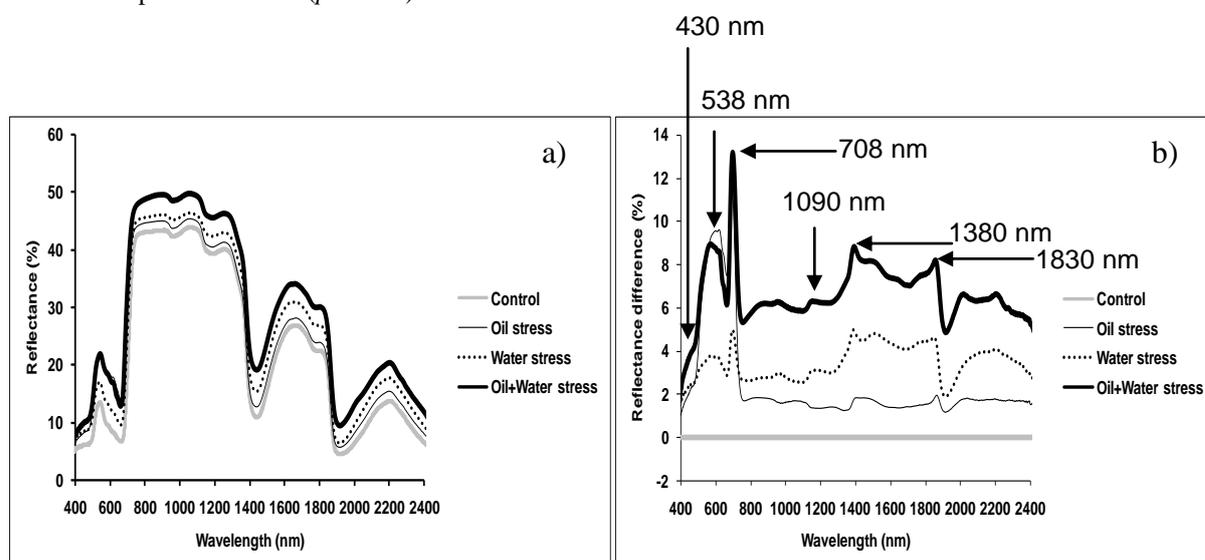
Figure 5. Spectral response to treatments, mean reflectance spectra (a), differences between the mean spectral reflectance (b) of the treated and control maize leaves 18 days after treatment. Treatments as denoted by the key,  $n = 100$ .
