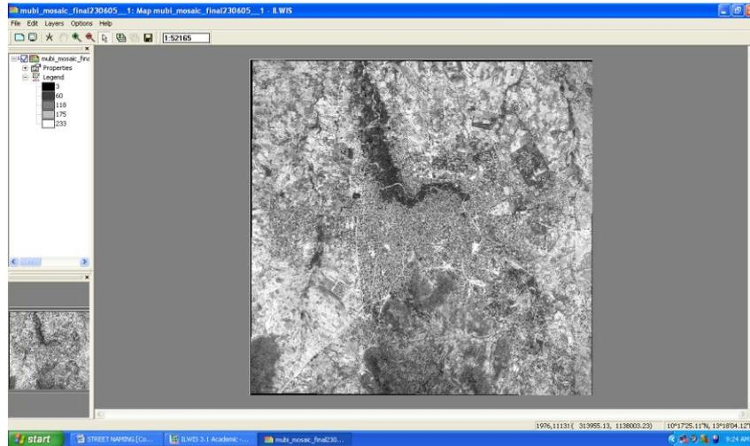
Figure 2: Georeferenced and resampled image of Mubi metropolis.
