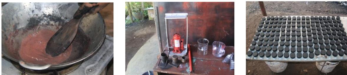
Figure 2. The process of making charcoal briquettes
