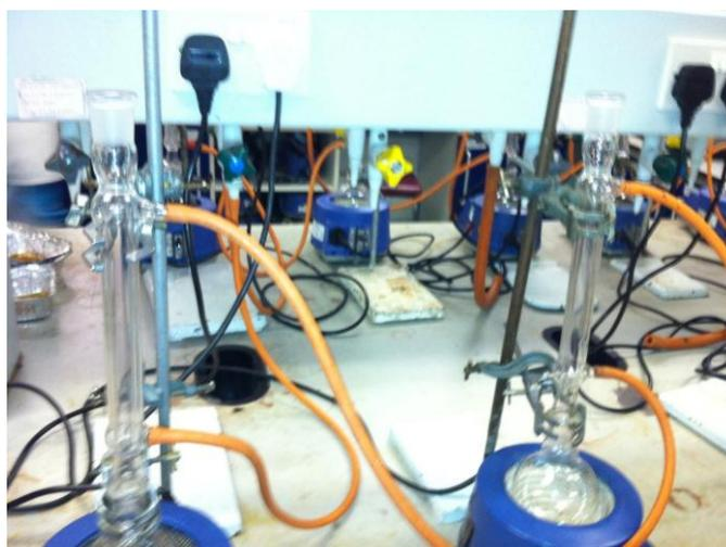
**Fig 7 Experimental setup for carbon content determination**
