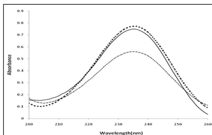
Figure 4. Spectrophotometric observation of crotonic acid peak at 235 nm, P(3-HB) from Aldrich (—); Metabolix MBX D411G (-----); P(3-HB) extracted from BP/SU1 cultivated in 53% WE mineral media . (· · ·)
