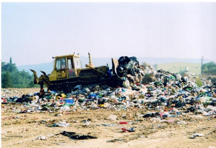
**Fig 1: A bulldozer compacting municipal waste freshly delivered to the sanitary landfill site of Temploni on the island of Corfu. In the distance; the new Materials Recycling Facility (MRF) for processing commingled recyclables can also be seen (Author's photo)**
