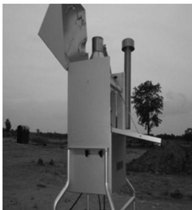
Figure 2.1: High Volume sampler installed at the proposed site
