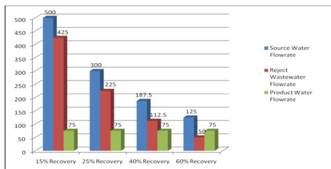
Figure 3. Wastewater Generation for Various Recovery Rates
