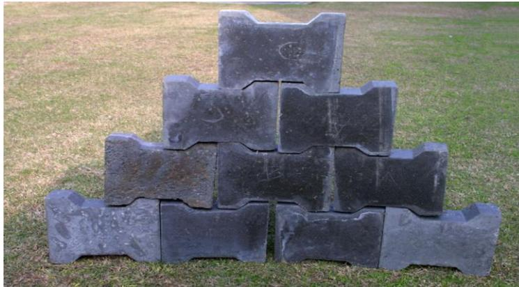
**Fig. 2:** Photograph of fabricated paving blocks at the age of 28 days
