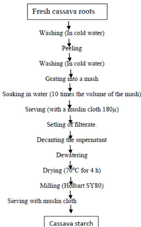
**Fig.1:** Flow chart for production of food quality starch.
