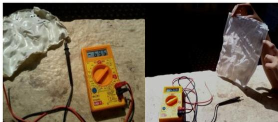
Figure no. 2 a) current generation by constructed solar panel b) Control: solar panel without thylakoids
