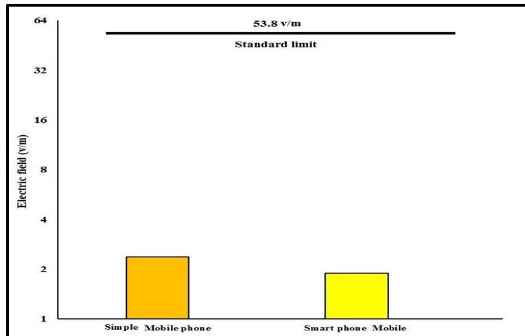
Figure 2. Comparing the Electric Field of Simple and Smart Phones with Standard Limits
