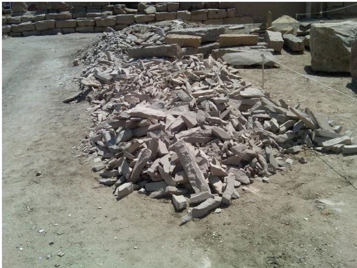
**Photo 15:** Scrap sandstone from a local mission recycled for exterior flooring
