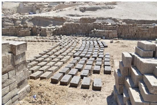
**Photo 12:** New mud brick drying in the sun with stacked dried specimens
