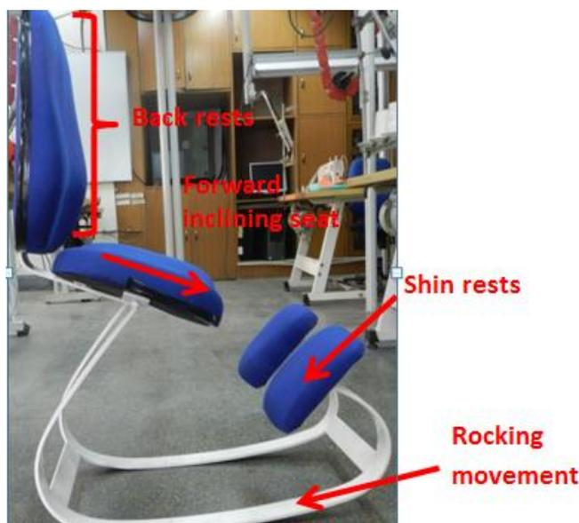
**Fig 7: Prototype of Chair C with inclined seat; padded shin rests and rocking feature**
