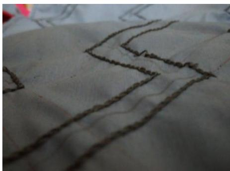
Figure 6: Close view of conductive thread trace
