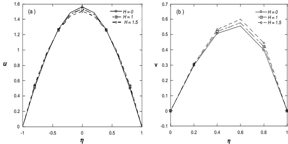
**Fig. 2.** Axial and normal velocity profiles for different values of  $H$ ;  $S = 1$  and  $Re = 1$ .
