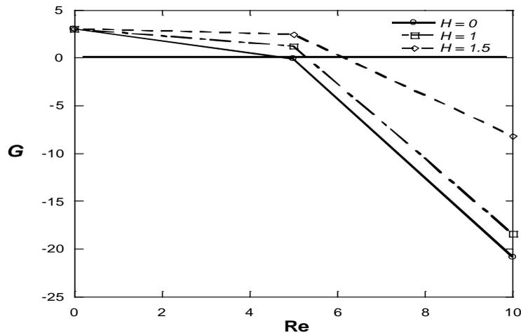
**Fig. 3.** Wall shear stress at  $S = 1$  for different values of  $H$ .
