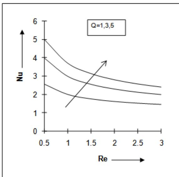
**Fig.9:** Nusselt number against  $Re$  for different  $Q$  when  $U=1, Gr=10, Gm=15, M=2, Pr=0.71, Sc=0.6, Sr=0.5, \epsilon=0.001$
