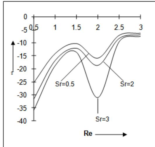
Fig.12: Skin friction against  $Re$  for different  $Sr$  when  $U=1$
