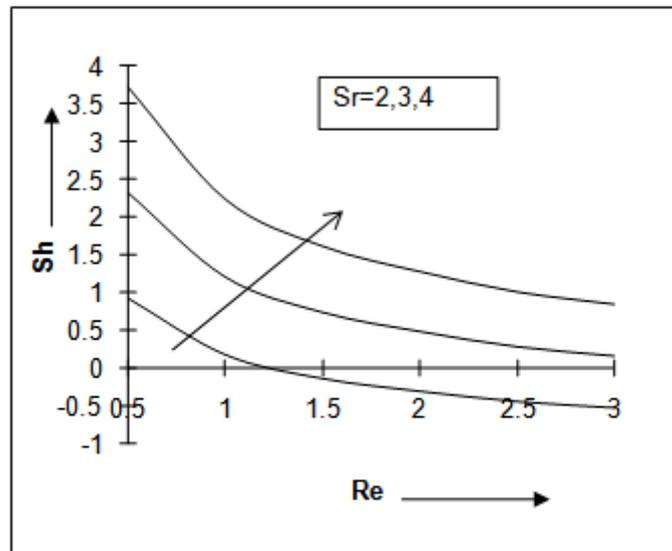
Fig.15: Sherwood number against Re for different Sr when Gr=10, Gm=15, M=2, Pr=0.71, Q=1, Sc=0.6,  $\varepsilon = 0.001$  K=1, U=1
