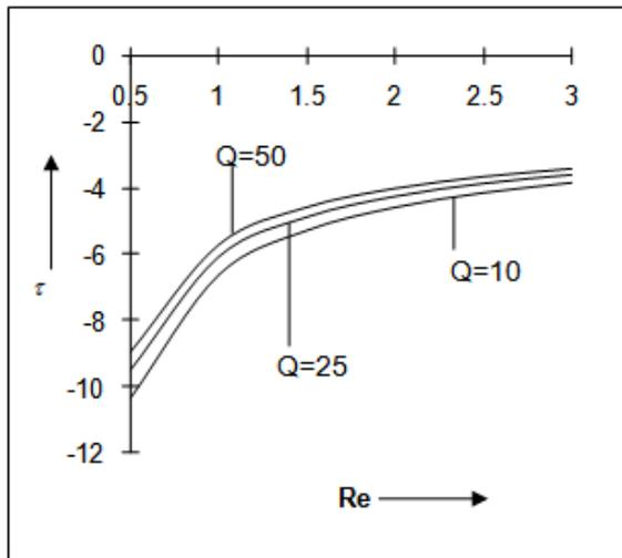
Fig.11: Skin friction against  $Re$  for different  $Q$  when  $U=1$
