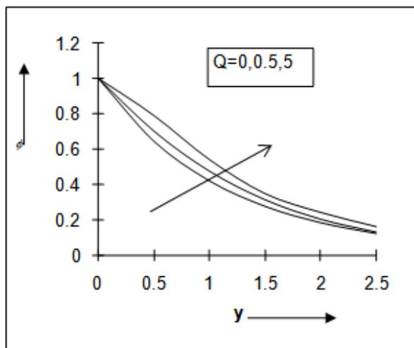
**Fig.7:** Species concentration versus  $y$  for different  $Q$   $Gr=10, Gm=15, Re=1, M=2, Pr=0.71, K=1, Sc=0.6, Sr=1, \epsilon=0.001$
