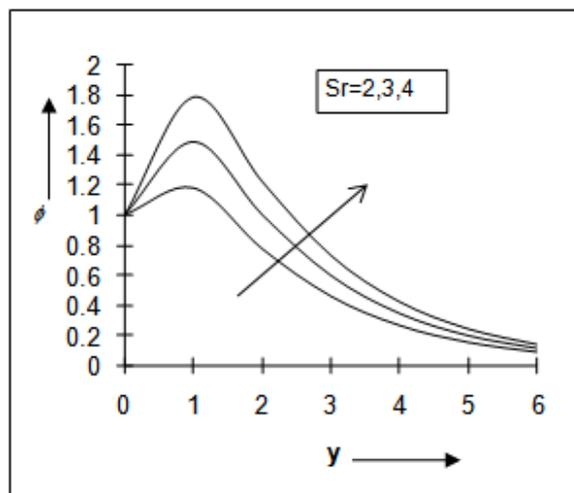
**Fig.8:** Species concentration versus  $y$  for different  $Sr$  when  $U=1, Gr=10, Gm=15, Re=0.5, M=1, Pr=0.71, K=1, Sc=0.6, Q=5, \epsilon=0.001$
