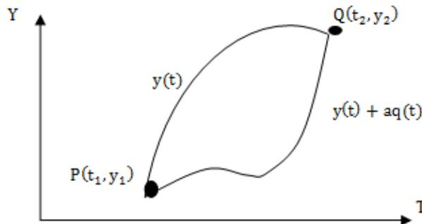
Let the original shape of the curve be  $y = y(t)$ . Suppose there is a small variation due to certain disturbance, the curve changes shape to  $y^*(t) = y(t) + aq(t)$ , where 'a' is a small parameter,  $q(t)$  is an arbitrary function,  $y^*(t)$  is the new curve,  $q(t_1) = 0$  and  $q(t_2) = 0$ , implies no variation in  $t$ . This means that
