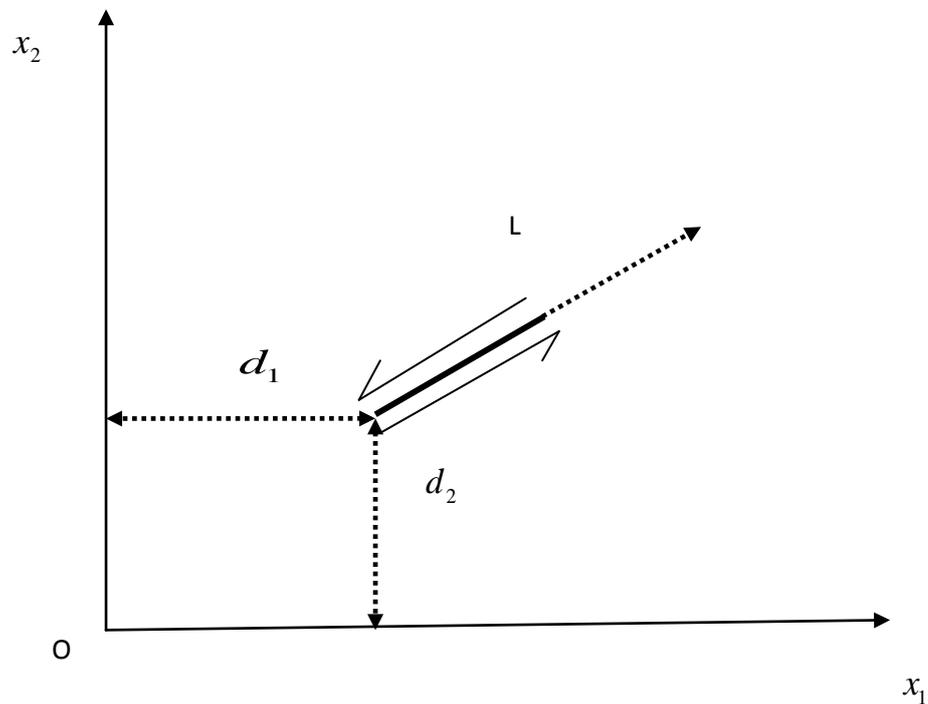
**Geometry of Strike-slip fault of width  $L$  at a distance  $d_1$  from  $x_2$ -axis and  $d_2$  from  $x_1$ -axis for the uniform monoclinic half-space**
