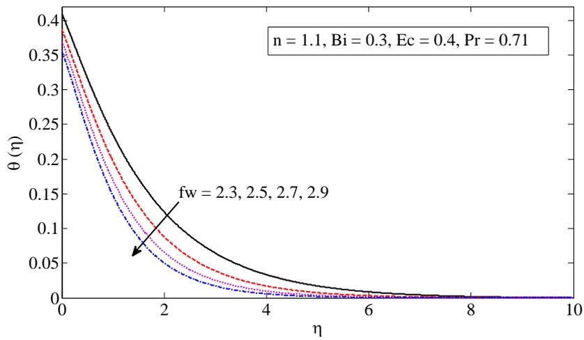
Fig.4 Temperature for various values of  $f_w$
