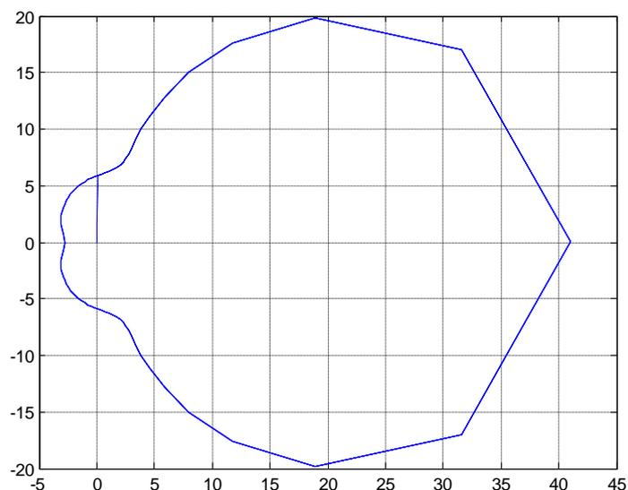
**Fig 3: Region of Absolute Stability for Block-Scheme K=3**
