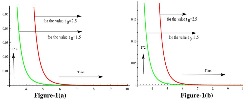
Figure-1(a), Figure-1(b) represents the energy decay of temperature fluctuation for four -point correlations of equation (38). When the Prandtl No. is small as of mercury  $P_r=0.015$  and  $\nu=0.1$  at  $20^\circ\text{C}$  Temp  $\nu=0.08$  at  $80^\circ\text{C}$  Temp. It is observed that the energy decays more rapidly as viscosity decreases from 0.1 to 0.08 at temp.  $20^\circ\text{C}$  to  $80^\circ\text{C}$ .
