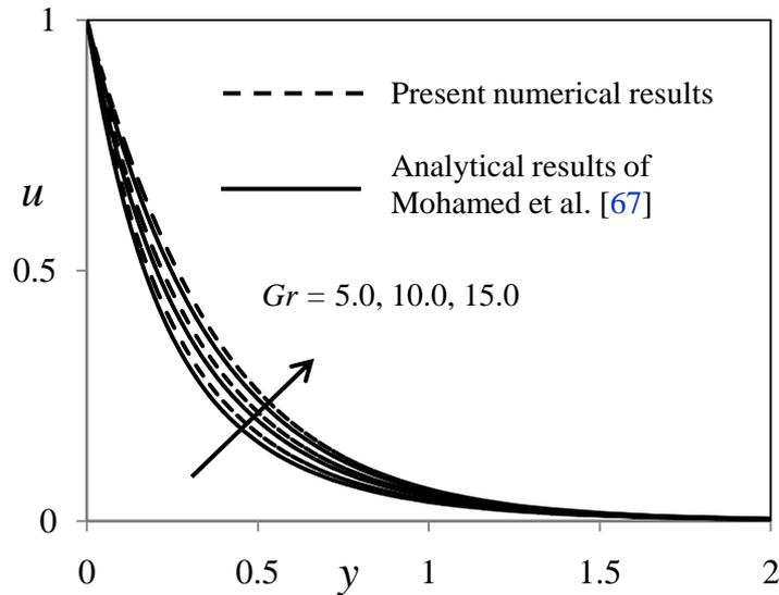
**Fig. 3.** Comparison between present numerical results with the analytical results of Mohamed et al. [67] for different values of  $Gr$  in absence of viscoelastic Rivlin-Ericksen fluid.
