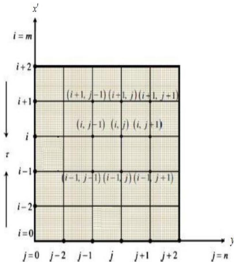
Fig. 2. Finite difference space grid
