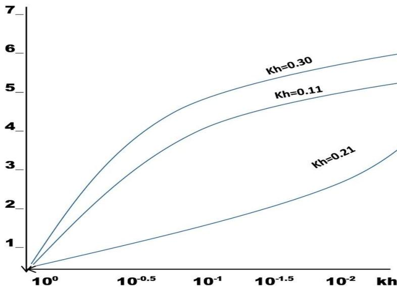
Fig. 3. Probability of exceedence for wave crest elevation (Period T=12secs, t= 5 mins)
