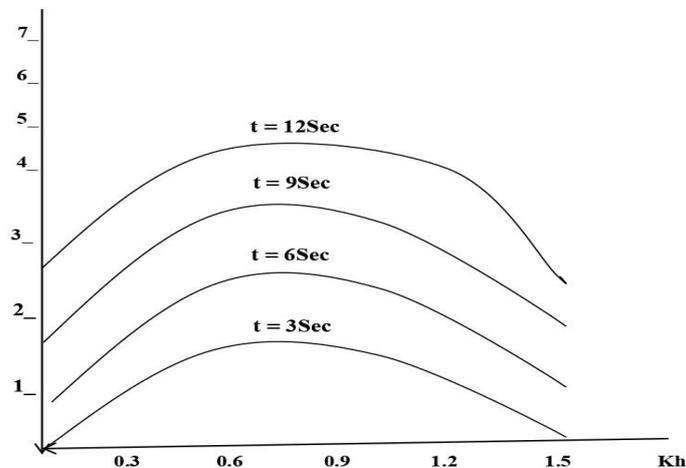
Fig. 1. The distribution of the maximum wave crest amplitude in the presence of a vertical wall
