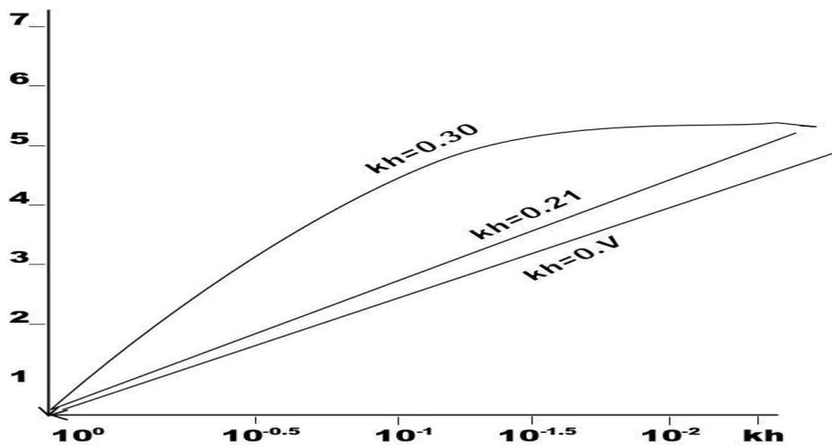
Fig. 2. Probability of exceedence for wave crest elevation (Period T=8secs, t= 5 mins)
