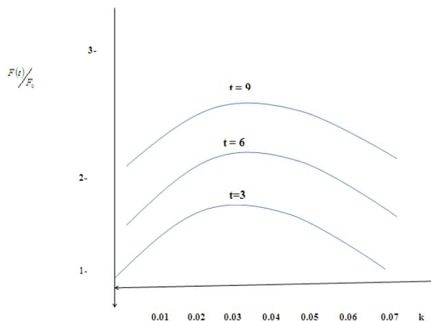
Fig.4. Fluctuating wave force in front of a vertical wall  $k = rad / min, F_0 = \rho g \sigma^2$
