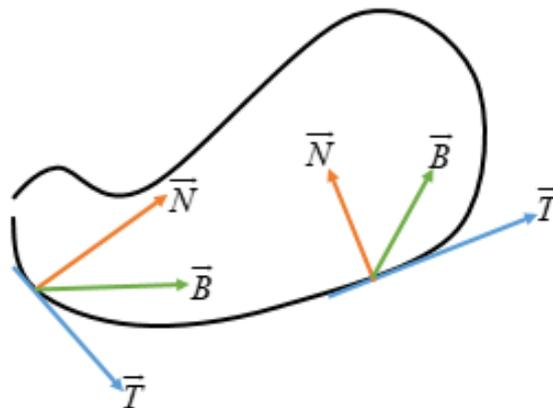
Figure 3: Moving Frenet frame
