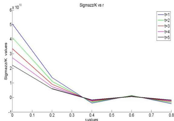
**Fig.5** Axial stress function  $\frac{\sigma_{zz}}{K}$  for thin plate ( $M=0$ ).
