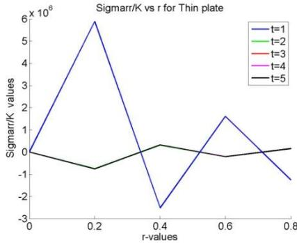
**Fig. 1** Radial stress function  $\frac{\sigma_{rr}}{K}$  for thin plate ( $M=0$ ).
