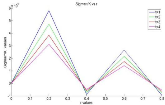
**Fig. 2** Radial stress function  $\frac{\sigma_{rr}}{K}$  for thick plate ( $M \neq 0$ ).
