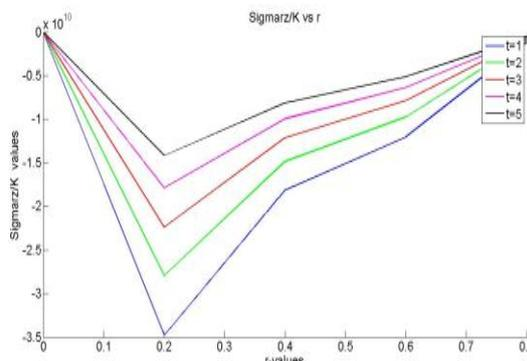
**Fig.8** Stress function  $\frac{\sigma_{rz}}{K}$  for thick plate ( $M \neq 0$ ).
