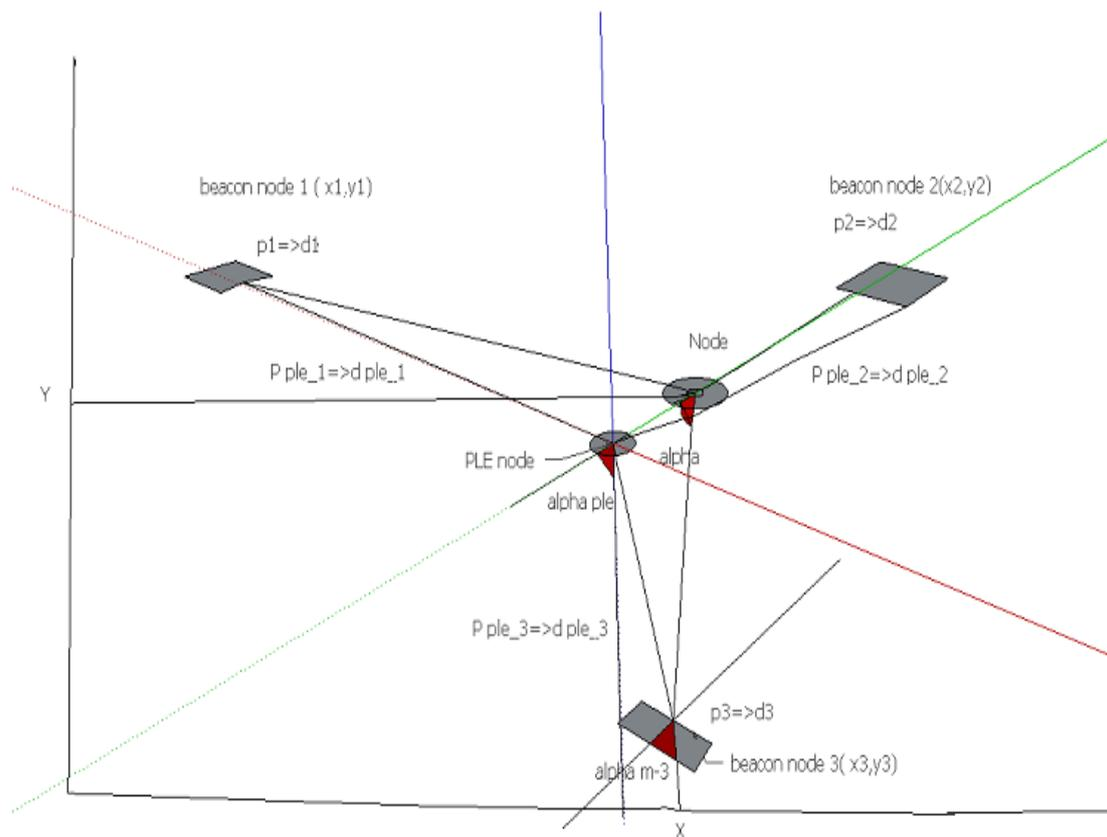
Figure 3: Geometrical diagram of localisation RSS PLE in 3D
