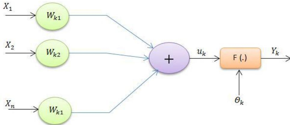
Figure:4 [4]. Model of artificial neuron
