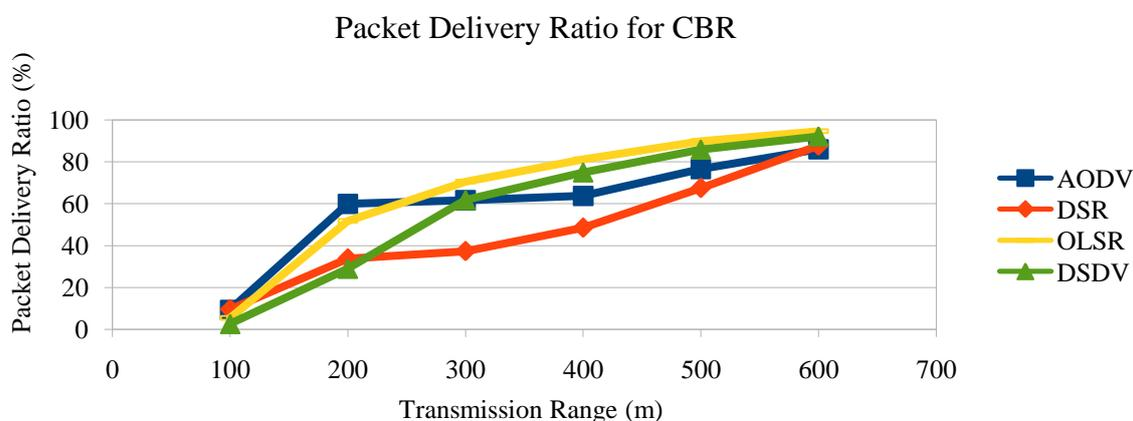
**Fig.21.** Packet Delivery Ratio Vs Transmission range
