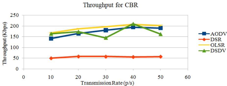
**Fig.19.** Throughput Vs Transmission rate
