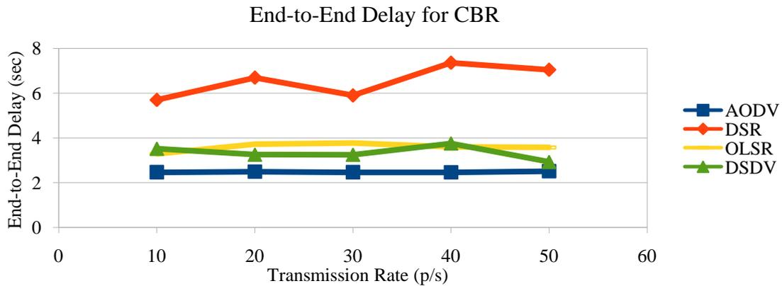
**Fig.18.** End-to-End Delay Vs Transmission rate
