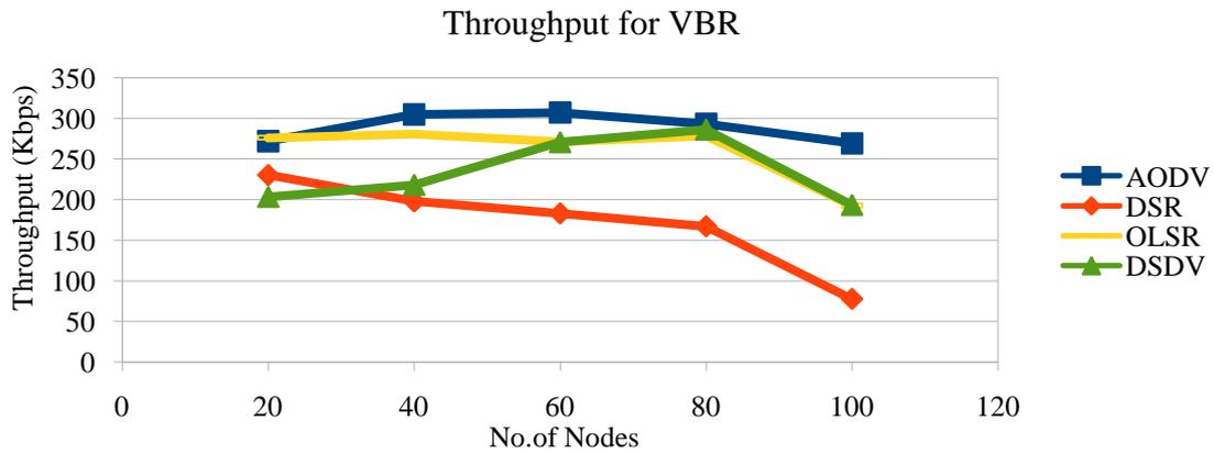
Fig.13. Throughput Vs Number of Nodes
