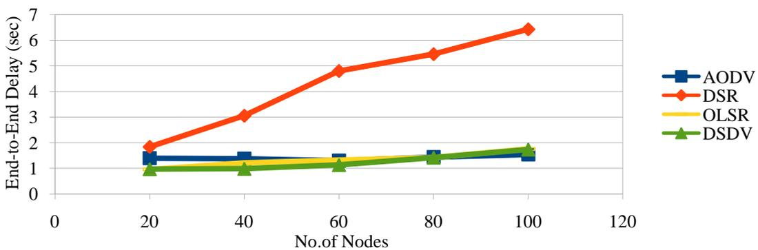
Fig.11. End-to-End Delay Vs Number of Nodes
