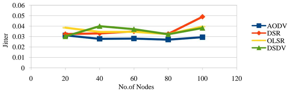
Fig.14. Jitter Vs Number of Nodes
