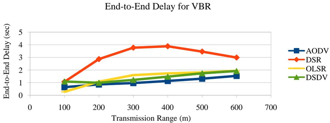
Fig.26. End-to-End Delay Vs Transmission range
