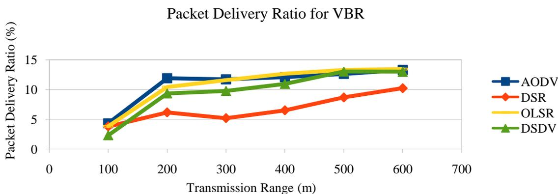
**Fig.22.** Packet Delivery Ratio Vs Transmission range
