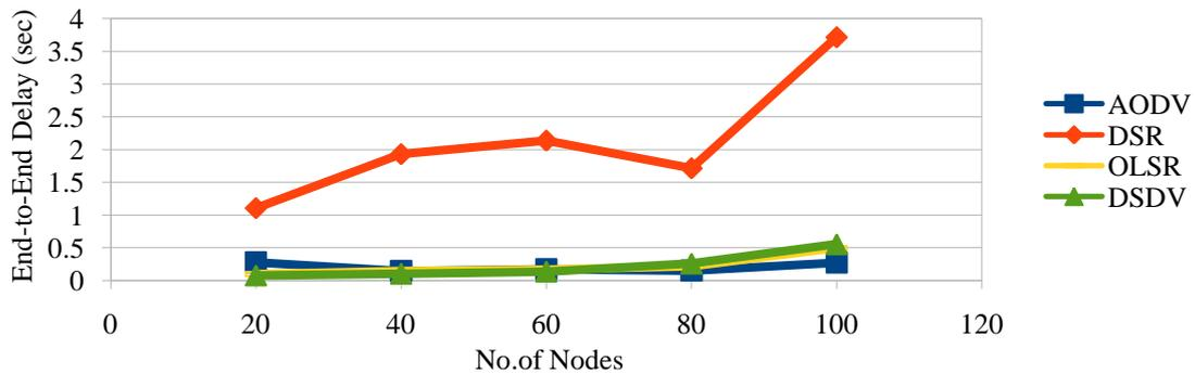
Fig.10. End-to-End Delay Vs Number of Nodes
