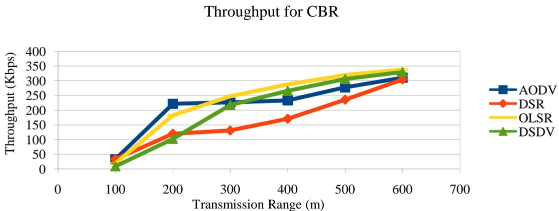
Fig.27. Throughput Vs Transmission range
