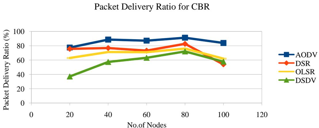
Fig.6. Packet Delivery Ratio Vs Number of Nodes
