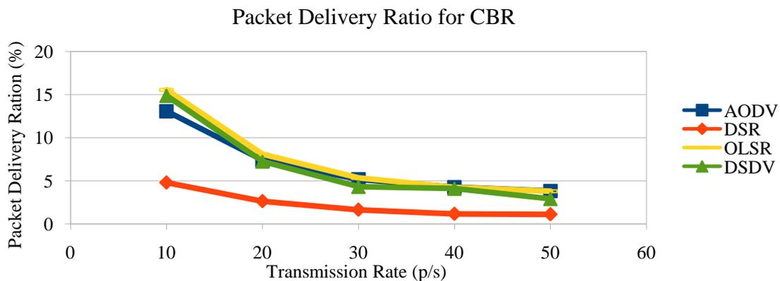
**Fig.16.** Packet Delivery Ratio Vs Transmission rate
