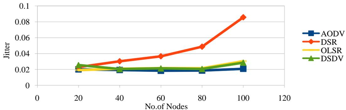
Fig.15. Jitter Vs Number of Nodes
