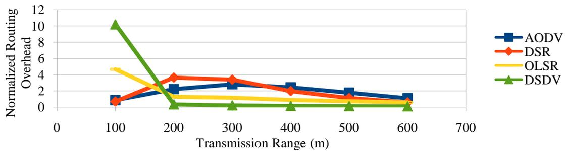
**Fig.24.** Normalized Routing Overhead Vs Transmission range
