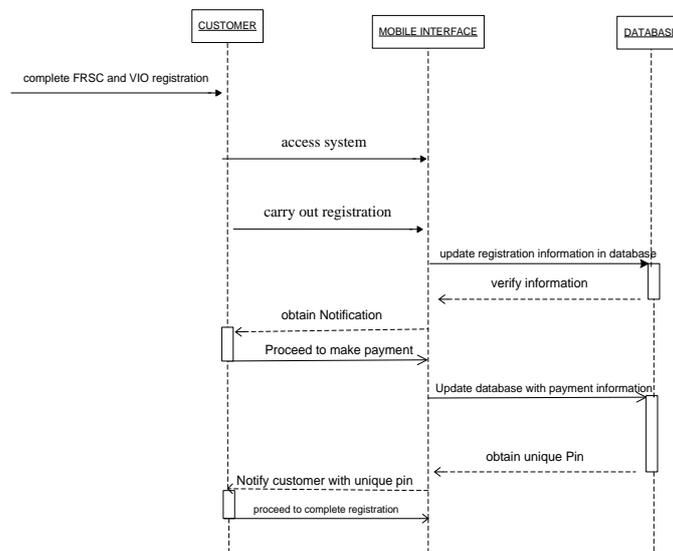
Figure 3: Sequence diagram of the proposed approach
