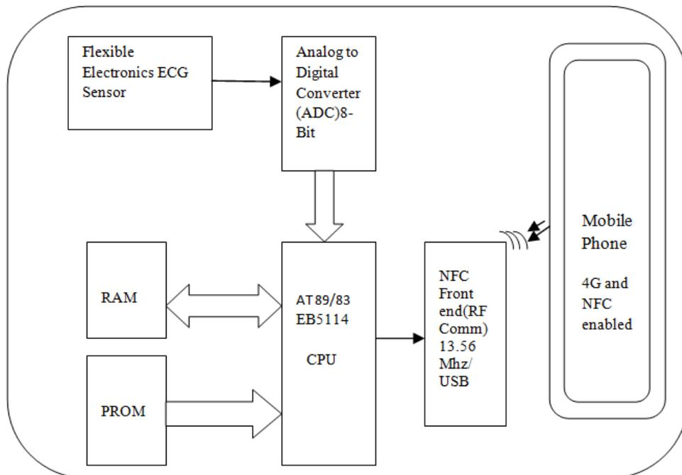
**Fig 3** Block Diagram of Body Area Electronics Dongle for Mobile Phone Communication
