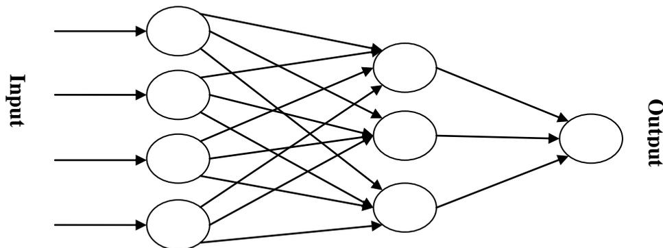
**Figure 1.** Architecture of neural network(Multi Layer Perceptron)
