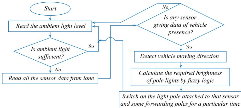
Figure no2: The algorithm of the intelligent streetlight system
