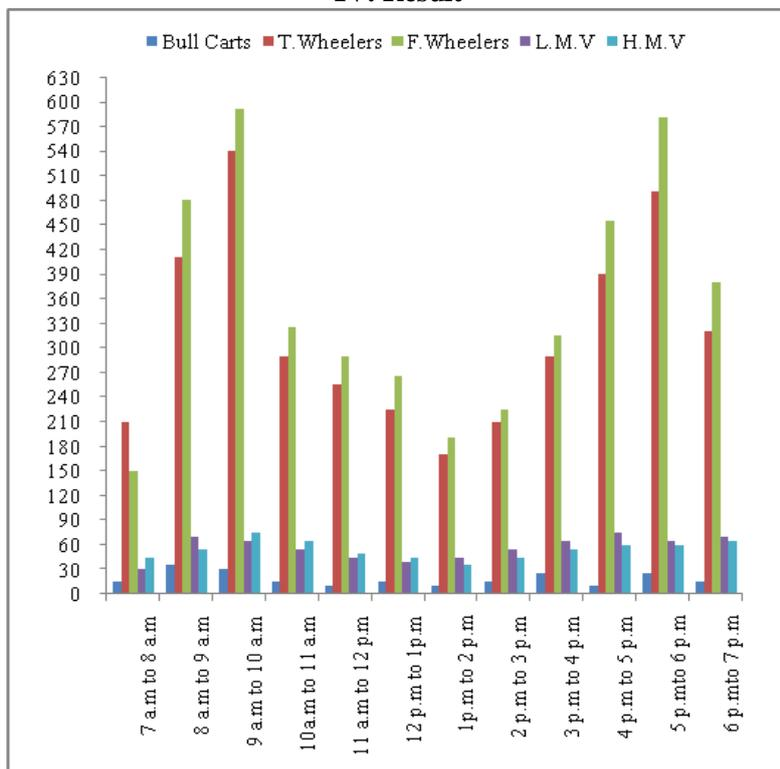
Fig.2. Traffic Volume Landran to Chandigarh (Peak Hour 9-10am, 5-6pm)
