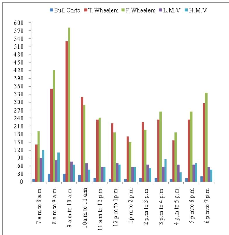
Fig.5. Traffic Volume Landran to Banur (Peak Hour 9-10am, 6-7pm)
