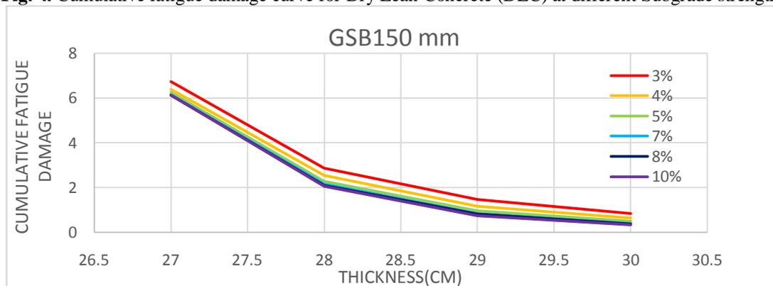
Fig.5. Cumulative fatigue damage curve for Granular Subbase (GSB) at different Subgrade strengths
