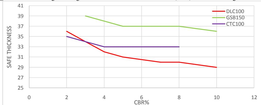
Fig.7. Safe thickness VS CBR% by IRC: 58-2002
