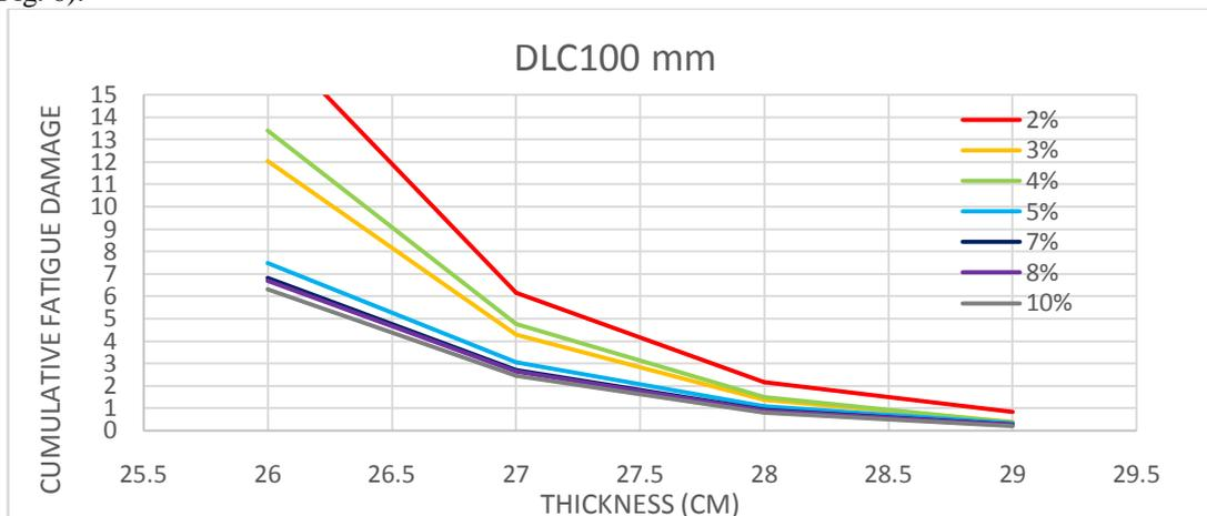
Fig. 4. Cumulative fatigue damage curve for Dry Lean Concrete (DLC) at different Subgrade strengths
