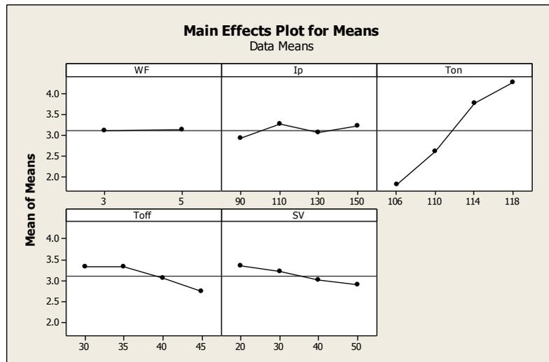
Fig. 2 Effects of response of Process Parameters on Cutting Rate (Raw Data)
