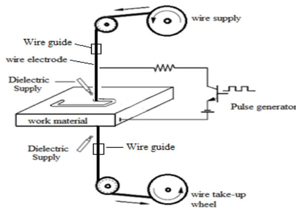
Fig. 1 Wire Electrical Discharge Machining (WEDM) process [12]
