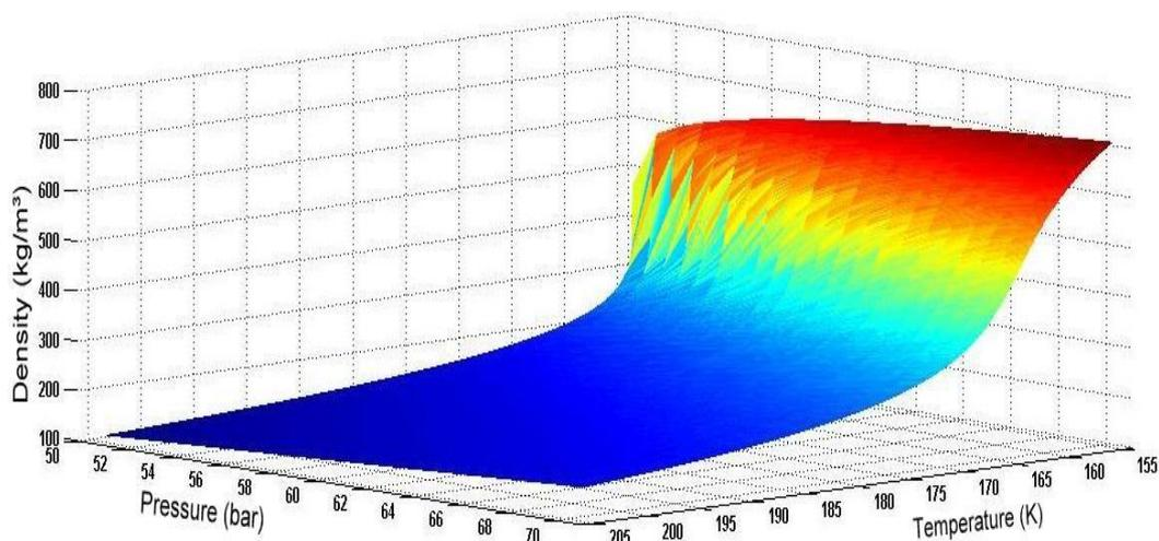
**Fig 2: Variation of Density as a function of temperature (154.58K-204.58K) and Pressure (50.43bar-70.43bar)**
