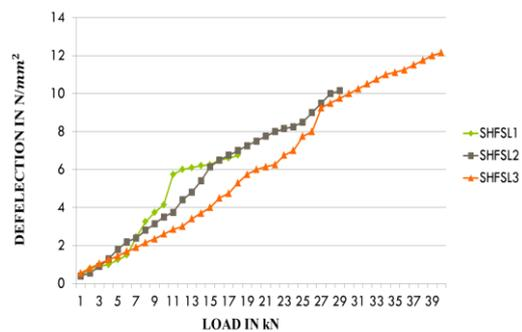
FIG.3.15 LOAD vs MIDSPAN DEFLECTION FOR STRENGTHENED SELF-COMPACTED FERROCEMENT SLABS WITH FIBRES
