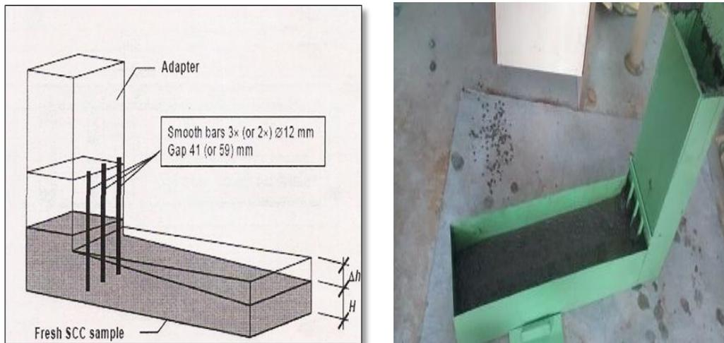
Fig 3.4 L Box Test Apparatus
