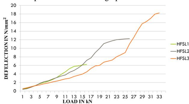
FIG.3.14 LOAD vs MIDSPAN DEFLECTION FOR SELF-COMPACTED FERROCEMENT SLABS WITH FIBRES
