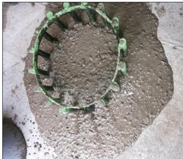
Fig 3.2 J-ring test apparatus
