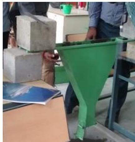
Fig 3.3 V-Funnel Test Apparatus
