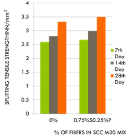
FIG.3.6: SPLITTING TENSILE STRENGTH RESULTS
