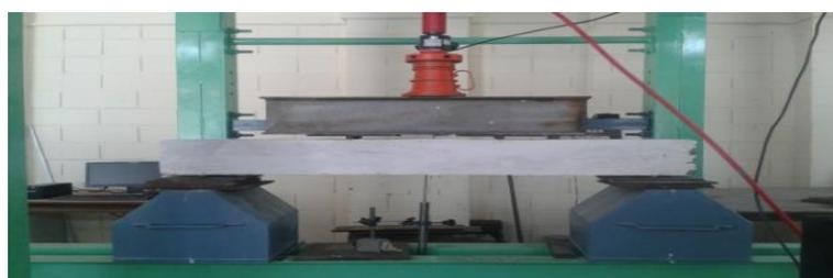
**6.5a Test set up for a beam**
