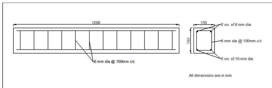
**6.2a Reinforcement details as per IS13920**
